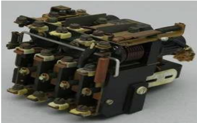
An example of the actual firing mechanism used on the Pylon to defend Sydney and its harbour. This is on display at the Powerhouse Museum's Castle Hill site.
