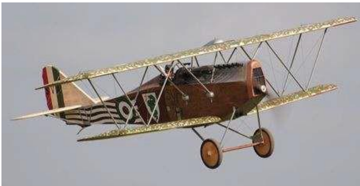
Warren truss designs were used in building aircrafts such as the Italian First World War aircraft Ansaldo SVA
